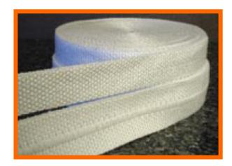
This is a widely used and universal tape for making gaskets, especially where a rough or uneven surface or flange exists. The tape is a fiberglass base with a special white rubber formulation. The tape is tacky, and has a plastic film surface covering that is removed before installation. The tape will stick to itself once the film is removed.
